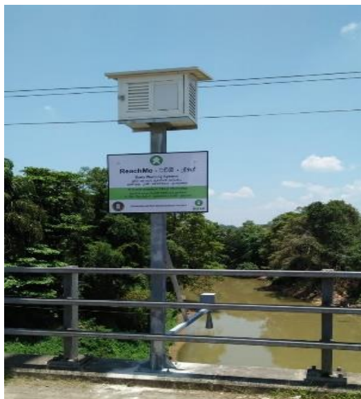
Figure 3. Sonar sensor installed to monitor Kalu Ganga in Ratnapura
