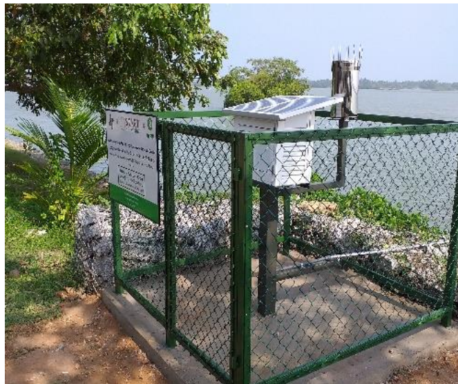
Figure 1. Water level monitoring sensors in Batticaloa
